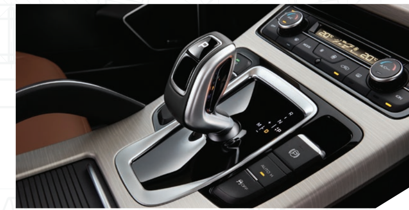
7-Speed Dual Clutch Transmission with Manual Mode
