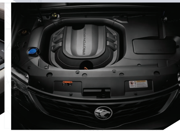
1.5L TGD i Engine Max Power: 177PS Max Torque: 255Nm
